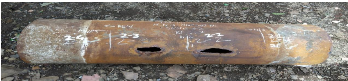
Corrosion Damage to the portion of pipeline
